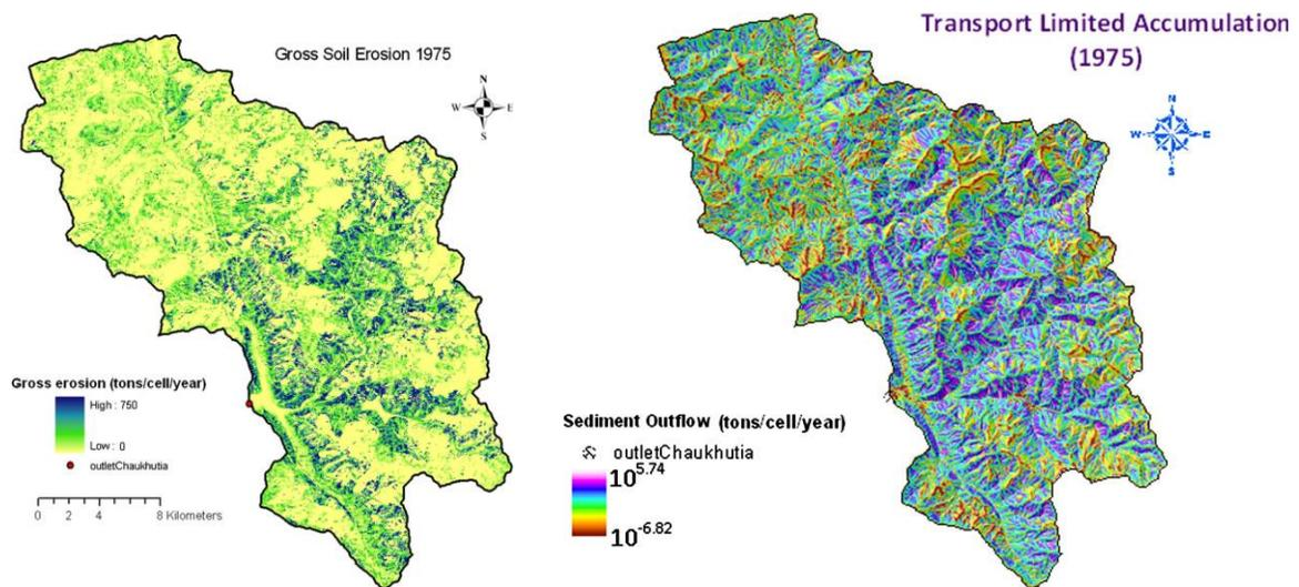
**Fig. 8:** Gross soil erosion map for the year 1975    **Fig. 9:** Transport limited sediment outflow for year 1975
